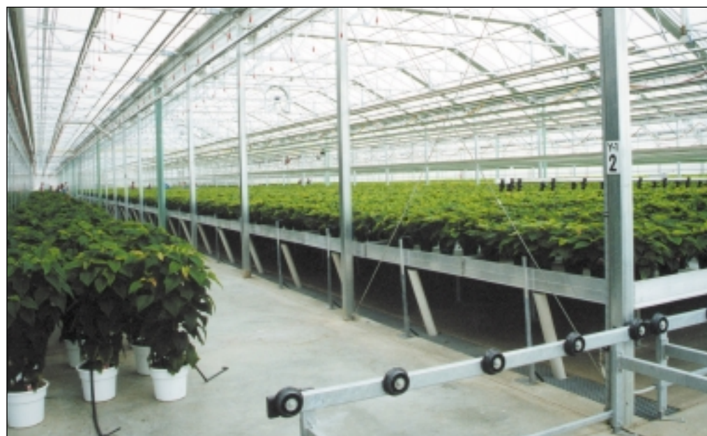
Plantpeddler's 2-acre facility is loaded with automation, including sticking lines, automated bench loading, continuous flow bench washer and an irrigation control center.
